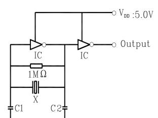
X: ZTAWS3.58MG IC: 1/6TC4069UBP x 2 C1=C2: 30pF±20% (Typical)
