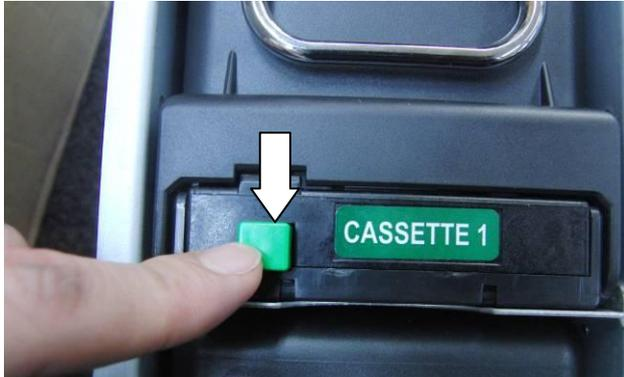
1) Pushing of LOKING PUSHER under CASSETTE , check whether the Lock is operated normally.
