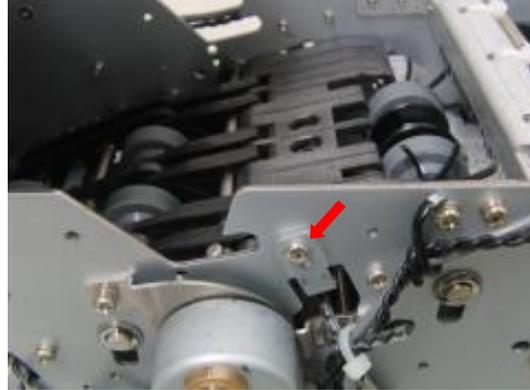
④ Pull sensor bracket out of the frame according to the picture.
