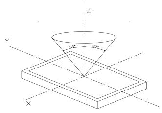
Inspection should be performed within angle  $\phi(\phi)$  is usually 30°) from Z axis to each X and Y. Inspection distance in any direction within  $\phi$  must be kept 30±5cm from the display surface.
