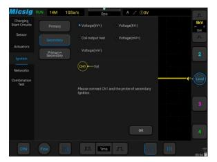
▲ The ignition system of a car is usually composed of primary and secondary coils and spark plugs.
