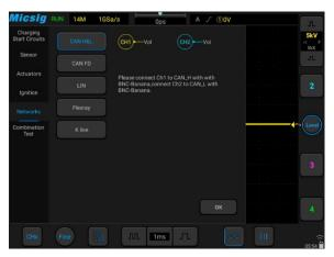
▲ SATO1000 is capable of acquiring and decoding CAN High /CAN Low, CAN FD, LIN, FlexRay, and K line signals, delivers professional Network communication tests on vehicles.
