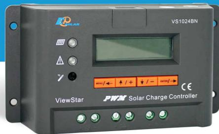
This Viewstar BN series is common negative controller, with LCD display, working data programmable, It has communication function via RS485 port to PC monitoring software, realizing real-time monitoring and battery management parameter setting.
