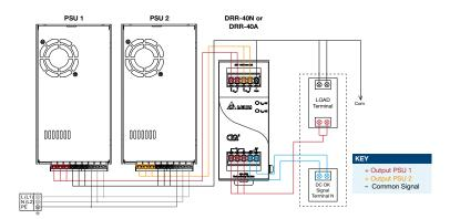
Fig. 5 Redundant Operation Connection Diagram
