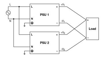
Fig. 6 Parallel Operation Connection Diagram
