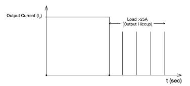
It is not recommended to prolong the duration of  $I_{\rm O}$  when it is <25A but >14.6A, since it may cause damage to the PSU.
