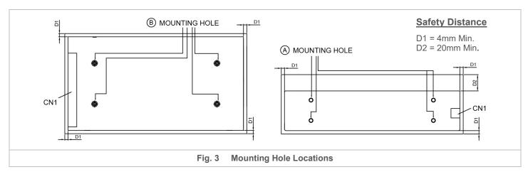
Ensure the mounted device is kept at  $\geq 4$  mm (0.16 inch) safety distance at all sides from other components and equipments. In addition, to ensure sufficient convection cooling, always maintain a distance of  $\geq 20$  mm (0.79 inch) from fan ventilated surfaces while the device is in operation. Please insert an insulation sheet between the system and product, if the safety distance is < 4mm (0.16 inch).
