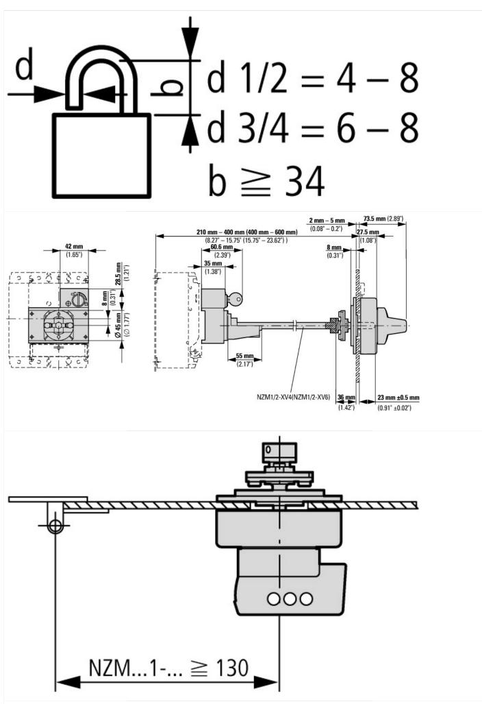
Minimum door coupling rotary handle clearance from door pivot point
