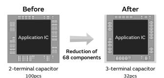
Reference: "How can the mounting area be reduced? —Methods of using low-ESL capacitors—"
