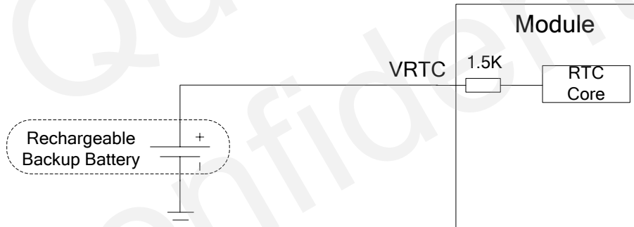
Figure 12: RTC Supply from a Rechargeable Battery
