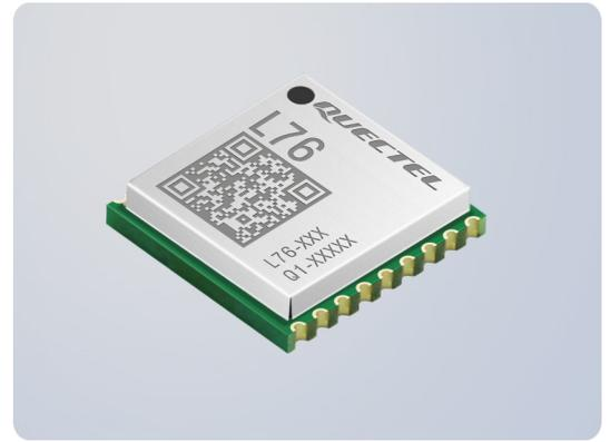
L76, the extremely compact GNSS module, is a concurrent GNSS receiver with multiple GNSS systems. It provides simultaneous GPS, GLONASS, Galileo, BDS and QZSS open service L1 reception capability. With 33 tracking channels, 99 acquisition channels, and 210 PRN channels, L76 can acquire and track any mix of multiple satellite signals.
