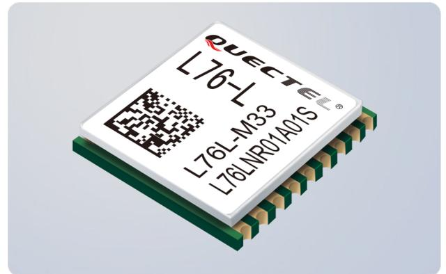
L76-L is a concurrent receiver module integrating GPS, GLONASS, Galileo and QZSS systems. With 33 tracking channels, 99 acquisition channels and 210 PRN channels, L76-L can acquire and track any mix of GPS, GLONASS and SBAS signals. Designed to be compatible with Quectel L76 module in the compact and unified form factor, L76-L provides a built-in LNA for better performance in weak signal areas.
