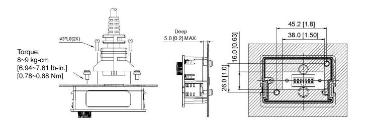
Method 2: Mounting through a plate (unit: mm [inch])
