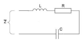
L: Ferrite core coil inductance R: Copper resistance and connection C: Tunning internal capacitor NPO Rdc: Optional parallel resistor Z: External impedance
