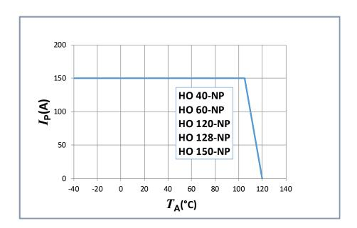
Important notice: whatever the usage and/or application, the transducer jumper temperature shall not go above the maximum rating of 120 °C as stated in page 2 of this datasheet.
