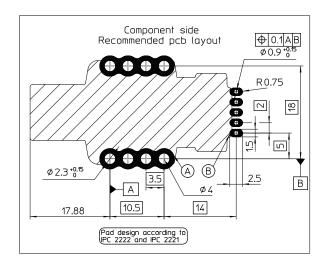
(Layout example with 4 jumpers in parallel)
