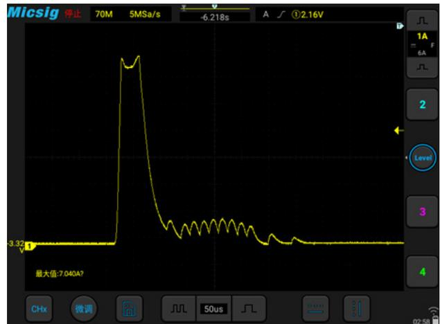
Surge current waveform at power adapter startup
