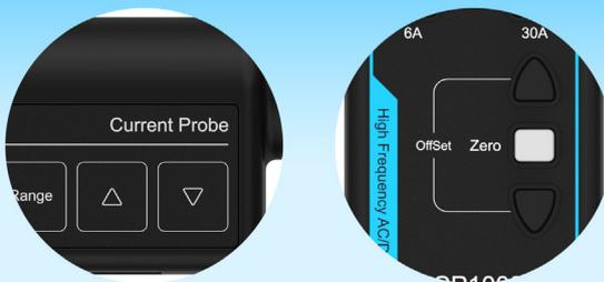
**CP503/CP1003:** Press the buttons "△" "▽" at the same time until the range LED green light turns off and then release, the probe will carry out Degaussing and Zero setting
