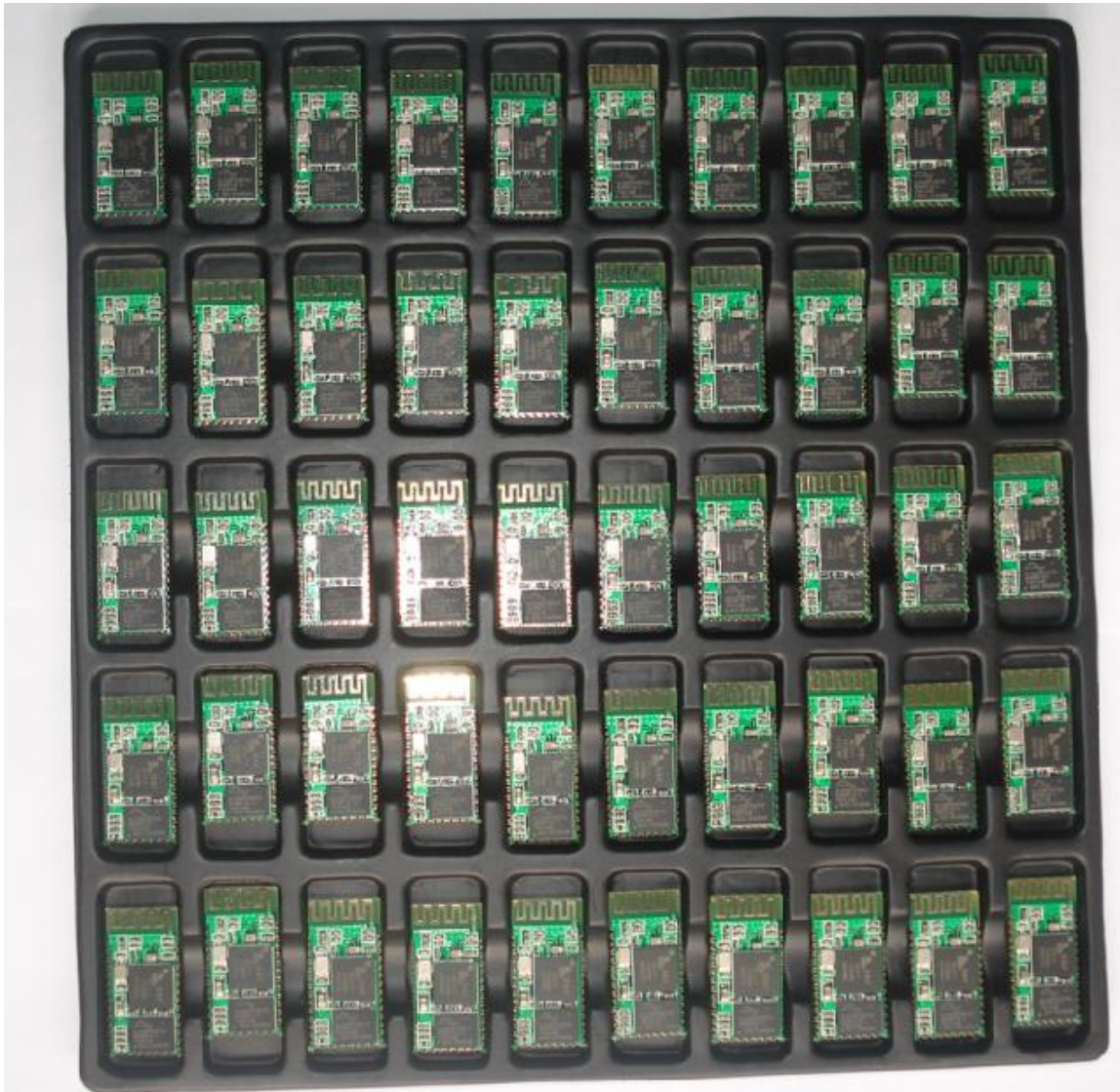
Figure 2 50 pieces chips in an anti-static blister package
