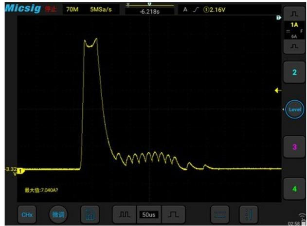
Surge current waveform at power adapter startup
