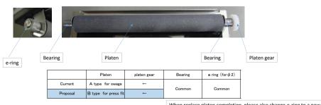
When replace platen completion, please also change e-ring to a new e-ring
