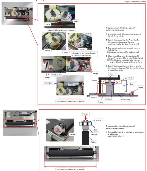
As mentioned above, on the gear of FTP-639CT004-R, since maintenance has many parts where the assembly by customer is difficult, correspondence of maintenance is not made. However, maintenance of the gear of platen becomes possible by changing platen completion. We propose the following.
