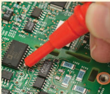
Reduce tip exposure for accurate placement
