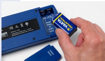
ET3 logger – replaceable battery
