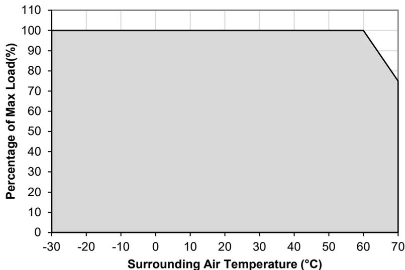
**Fig. 1 De-rating for Vertical Mounting Orientation**
