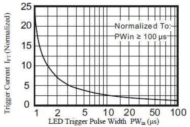
Fig.4 Current Required to Trigger VS Pulse Width
