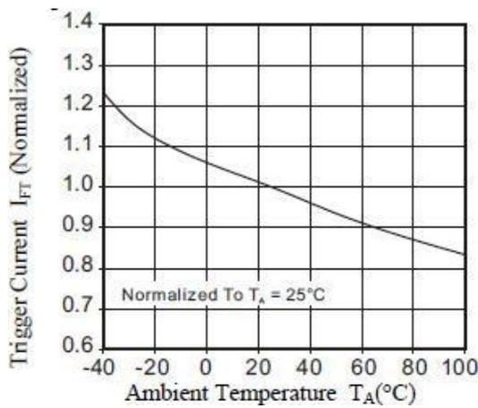
Fig.3 Trigger Current VS Temperature
