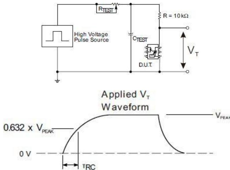
**Fig. 12. Static dv/dt Test Circuit & Waveform.**
