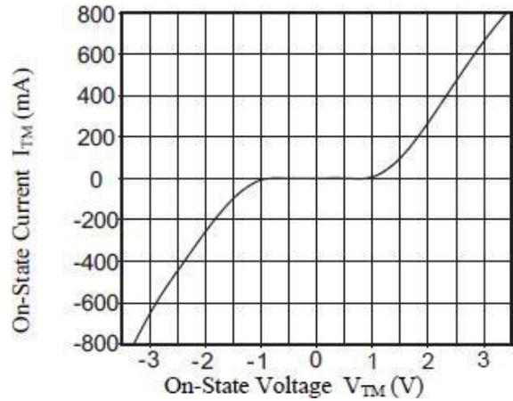
Fig.2 On-State Characteristics
