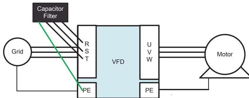
**Capacitive filter and drive wiring figure :**
