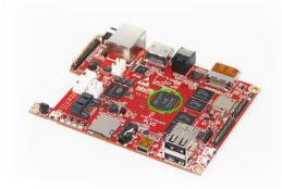
Allwinner H8 Octa-Core Cortex-A7 CPU @ up to 2.0GHz PowerVR SGX544 GPU @ up to 700MHz
