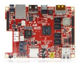
Cubieboard5 is the 5rd generation product of CubieBoard series from Cubietech Limited Company, and it's the updated version of CubieBoard3. Thanks to Allwinnertech' H8 SOC, Compared with CubieBoard3 the performance has been increased by 4 times. CubieBoard5 is open source hardware, single board computer, or development board which targets Developers, Geeks, Makers, Students...
