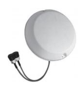
The CMD69273P, using patent-pending technology, is an indoor broadband low PIM 2-port MIMO omnidirectional ceiling mount antenna. It is designed to provide pattern coverage optimized for indoor requirements at 698-960 MHz and 1710-2700 MHz frequency bands. The individual antenna elements are designed with linear H/V-polarization components oriented to radiate a pattern that has been specifically shaped to deliver optimal performance from a ceiling mount location.
