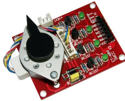
It is MINI Board Set to test STEPPING MOTOR that has been improved to interface with power supply to drive external STEPPING MOTOR; moreover, there is a particular Power Supply to drive Stepping Motor . It uses IC No.MC34063 and 4-Coil STEPPING MOTOR. It uses 4 of TR BC337 with LED to display the operating status and indicator to show directional rotation of Connector PIN HEADER 6 PIN.
