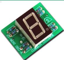
It is circuit of 7-Segment Red 1 Digit with R circuit connect with 7-Segment INPUT 10 PIN FEMALE and be able to connect with PORT I/O 10 PIN ETT directly.
