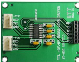
It is experiment or connect with RS232 circuit. Be able to use Power Supply VCC 3V to 5VDC and be able to connect RS232 2 channel 4 PIN ETT HEADER MALE 6 PIN AND FEMALE 6 PIN. Use IC DRIVER NO.ADM3232 OR other replaceable number.
