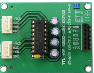
It is experiment or connect between RS232 with VCC 5VDC / 2 channel RS232 4 PIN ETT PORT HEADER MALE 6 PIN and FEMALE 6 PIN uses IC DRIVER NO.MAX232.
