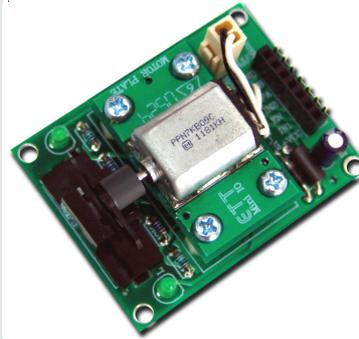
It is experiment of DC MOTOR Circuit with OPTO INPUT SENSOR 2 channel. It uses to test direction of rotation and speed of DC MOTOR with detected fan blade. It uses IC NO.L293D for DC MOTOR and PORT INPUT 7 PIN MALE/FEMALE.
