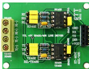
It is experiment or connect with RS422/485 circuit by using IC 75176 x 2 and connecting in RS422 or RS485 Type with Jumper. Be able to set PORT HEADER MALE 5 PIN and FEMALE 5 PIN.
