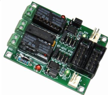
It is MINI Board version from ETT that uses 2 mini LOW POWER RELAY Circuits on board.
