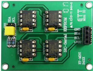
It is experiment of I2C by using 2 KBYTE IC EEPROM NO.24LC16 4 CHANNEL and be able to use in different point of I2C PORT HEADER MALE 4 PIN and FEMALE 4 PIN.
