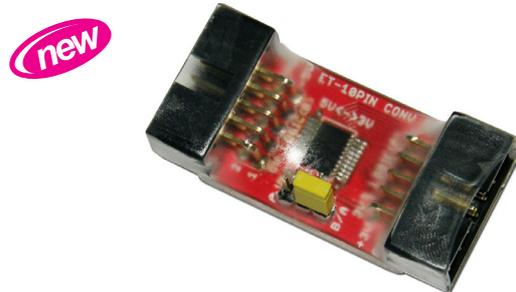
It is small board with 2 Connector 10PIN ET BUS I/O; it can be interfaced with 10PIN PAIR Cable conveniently. It is used to interface Circuit Signal LOGIC between 5V device and 3.3V device by using IC 74LX245 to be intermediate. It can set all 8BIT JUMPER. It can send data from 5V to 3.3V or from 3.3V to 5V, including Circuit 3.3V REGULATOR. It is suitable for Board MCU 3.3V I/O that is interfaced with Board 5V I/O.
