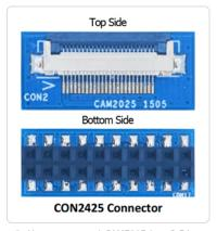
Or You can connect CAM500B to a 2.54 mm pitch double row interface with our CON2045 connector.
