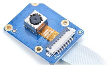
The CAM500B is a camera module using Omni Vision's  $\frac{1}{4}$ " QSXGA CMOS OV5640 chipset. It has a DVP parallel interface. It supports up to 5M-pixel (2592 x 1944) image sizes and 720P@30fps video recording. It supports various auto functions like AFC, AWB, AEC and etc.
