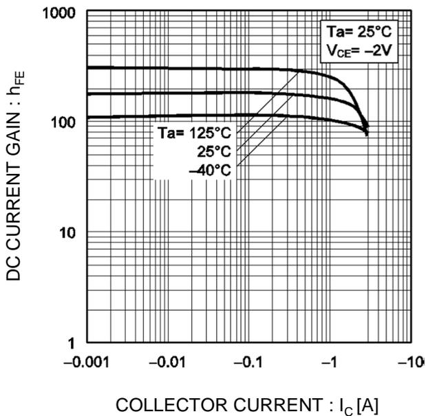
Fig.4 DC current gain vs. output current (II)
