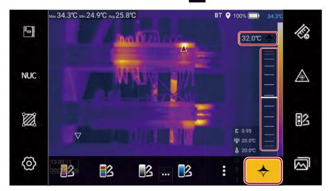
Figure 9. High Temperature Color Alarm
