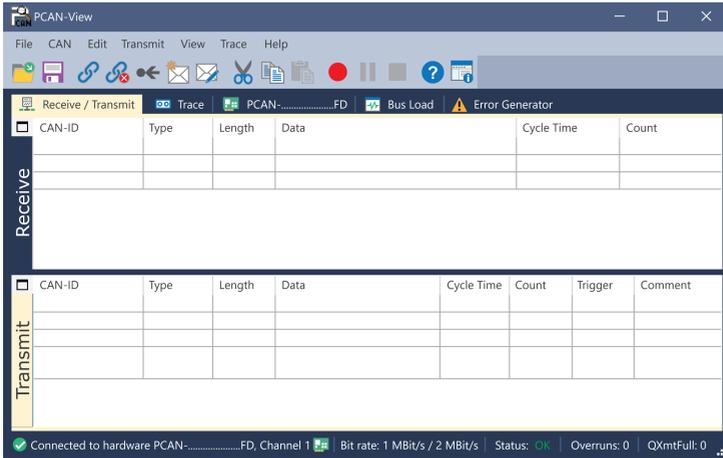
5. For initializing another channel or CAN interface, open another instance of *PCAN-View*.
