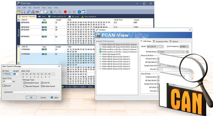
The CAN monitor PCAN-View is a Windows software for viewing, sending, and recording CAN and CAN FD messages. The software is installed with the installation of the device driver package under Windows.
