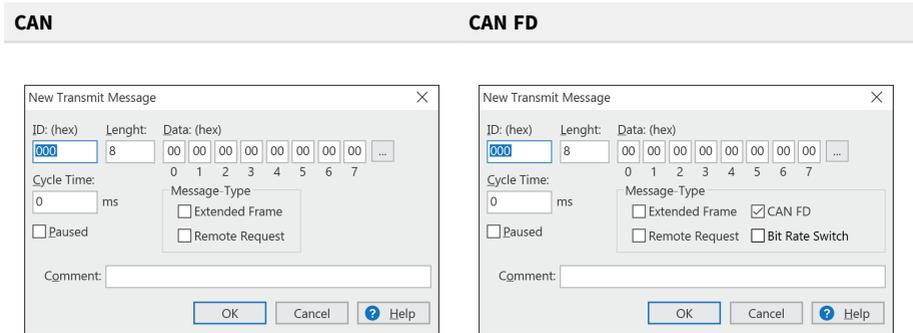
1. Enter the *ID*, *Length* and *Data* of the message. Other settings can be made according to the connected CAN bus.
