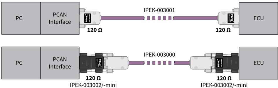
This example shows a connection between the PCAN Interface and a control unit (ECU). The upper example shows a connection with a cable which is terminated with  $120\ \Omega$  at both ends. At the lower example the connection is made with termination adapters.
