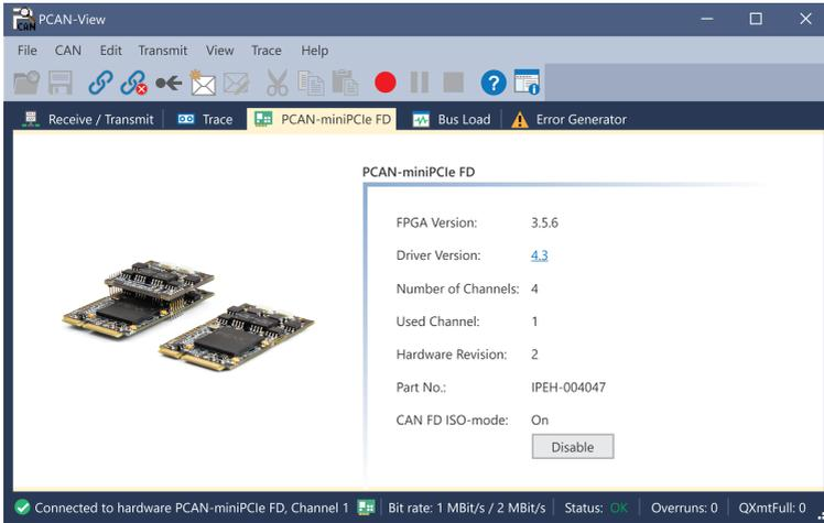
The *CAN interface* tab shows information about the hardware and the used Windows device driver. In this case exemplary for the PCAN-miniPCle FD. Depending on the CAN interface, a hardware ID can be determined to distinguish several interfaces of the same type. For interfaces with CAN FD a transmission according to "ISO" or "Non-ISO" can be set as default of the hardware.
