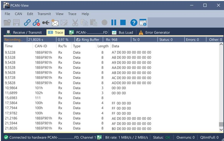
The tracer (data logger) records the communication of the CAN bus in linear or ring buffer mode. The trace data can be saved to a file.
