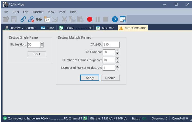
Via the *Error Generator* tab the communication on the CAN bus in test environments or during the development of CAN buses can be disturbed in a controlled way by 6 consecutive dominant bits. This is a violation of the CAN protocol on the CAN bus which must be recognized as an error by the connected CAN nodes.
