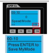
2. The parameter (Pr) displays in My mode if it is properly saved. To correct or to delete this parameter, press F4 for DEL.
