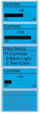
Press the Up / Down keys to adjust the setting value.
