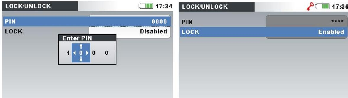
Figure 3.75: Lock/Unlock screen
