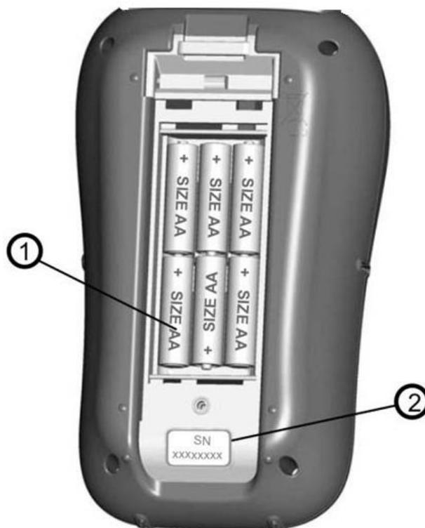
Figure 7.1: Battery compartment
