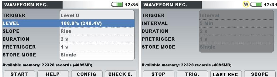
Figure 3.48: Waveform recorder setup screen
