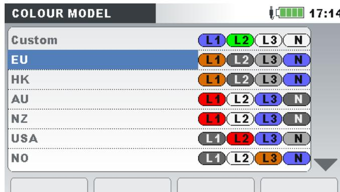
Figure 3.77: Colour representation of phase voltages
