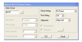
Click [...]. In the **Refer Device** dialog box, choose the VFD communication port that you need. If you want to read the output frequency (H), set the **Absolute Addr.** to 2202. For other values, refer to the ACMD Modbus Comm Address List (see Pr.09-04 in Chapter 12 Group 09 Communication Parameters).
