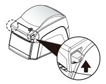
Turn off the printer and open the upper cover by pushing the knob in the direction of the arrow.
