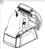
Insert paper roll into the printer.
