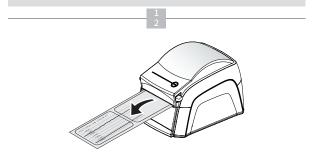
The printer is going to print out the media with the graph indicating how calibration is done for the sensor. This information will be automatically saved to ensure the accuracy on the form alignment. Once the graph is printed, cycle the power to get back into to READY mode.
