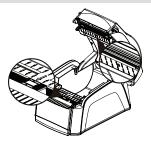
Black Mark Sensor and Notch sensor must always point to the same number.
