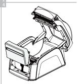
Assemble the cutter module to the correct position.
