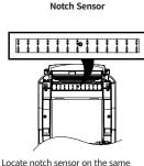
Locate notch sensor on the same number point- as the black mark sensor is indicating on.
