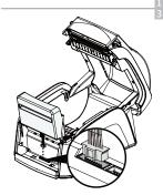
Connect the cutter connector to cutter position.
