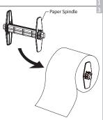
Pull out one of the adjustable width tabs. Insert a paper roll and adjust the tab so that the paper can be positioned in the center.
