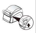
Turn off the printer and open the upper cover by pushing the knob in the direction of the arrow.
