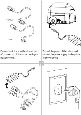
Connect the AC power cord to the power supply
