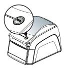
Press the "FEED" button and release immediately after the first beep.
