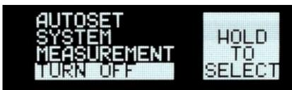
Figure 1-3: Turning off Display
