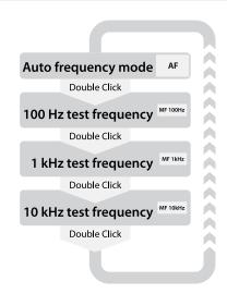
Figure 2-2: Selecting testing frequency
