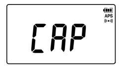
If you press  $\bigcirc$  ADJ without the included sensor cap attached to the illuminance sensor (when the count is equivalent to 1 lxor greater), [CAP] will be displayed on the LCD display. Press  $\bigcirc$  ADJ again after attaching the
