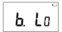
When the charge is gone, **[b. Lo]** blinks in the display for 3 seconds and the power is shut down automatically.
