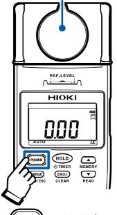
6 When the measurement is finished, put the sensor cap on and turn off the instrument.
