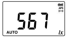
The auto range measurement starts when the instrument power is turned on.
