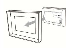
Tighten the screws with the torque less than 0.5 N-M / 0.7 N-M to avoid damage to the plastic Torque for DOP-112MX / 112WX / 115MX /
