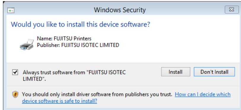
4. Connect the printer to the computer and switch on the printer. When the printer power on, it will install the DL3100 driver automatically. When the installation is finished, click “ok”.
