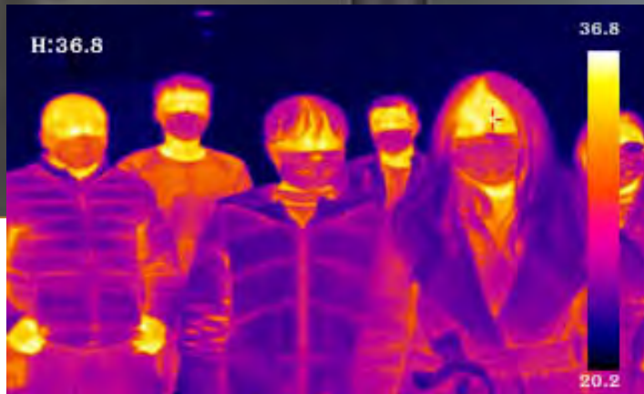
High temperature alarm with sound and tracking red cross mark.
