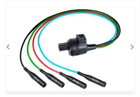
The adapter is attached to the test plug, after which earth electrodes, auxiliary earth electrodes, probe and auxiliary probe can be connected to the banana plug sockets at the test instrument.
