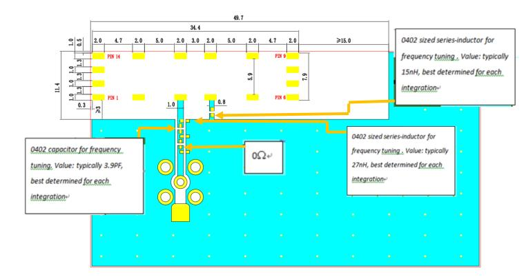
The antenna requires a matching circuit that must be optimized for each product. The matching circuit will require up to six components and the following circuit should be designed into the host PCB. Not all components may be required but should be included as a precaution. The matching network must be placed close to the antenna feed to ensure it is more effective in tuning the antenna.
