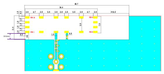
**Gap D** is required from the edge of the antenna to the ground plane. This should be maintained along the edge of the antenna placement, **minimum value is 3 mm**.
