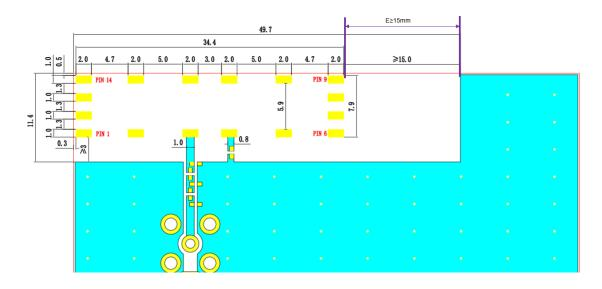
**Gap E** is required from the edge of the antenna to the ground plane or PCB traces, **minimum value is 15 mm.**
