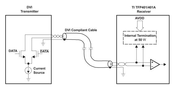
Figure 15. TMDS Differential Input and Transmitter Connection
