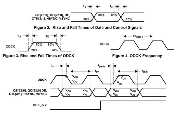
Figure 5. Data Setup and Hold Times to Rising and Falling Edges of ODCK
