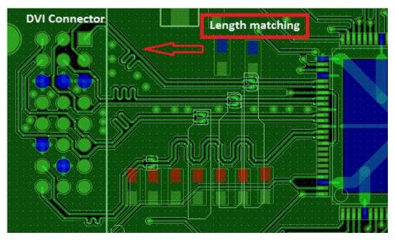
Figure 25. DVI Connector Routing
