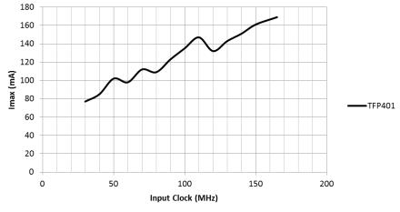
Figure 1. Imax vs Input Frequency
