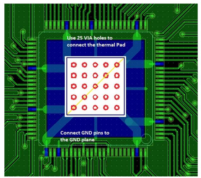
Figure 27. Ground Routing
