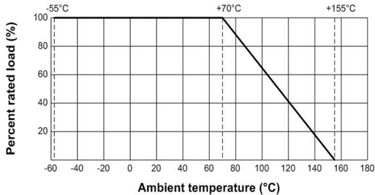
**Thin Film Chip Resistors (Terminal Lead Free)**
