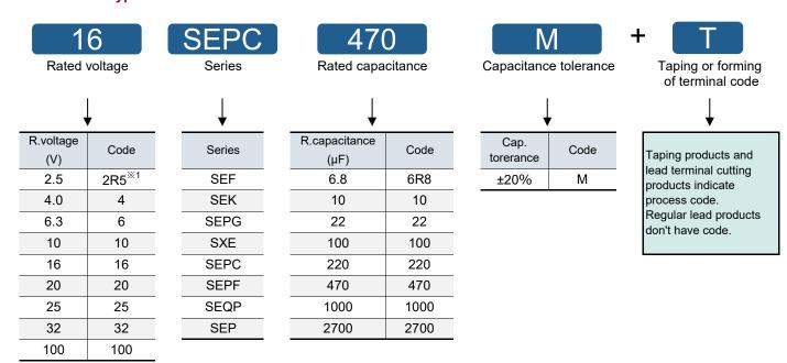
X1 Code 2 is used for 2.5 V products of B9, C6, C9, E7, E9 and F13 size in SEPC series.
