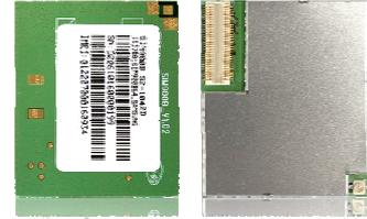
SIMCom presents a compact and reliable wireless module-SIM900B which is compatible with the module-SIM300/340 and SIM340E. This is a complete Quad-band GSM/GPRS module in a B2B type and designed with a very powerful single-chip processor integrating AMR926EJ-S core, allowing you to benefit from small dimensions and cost-effective solutions.
