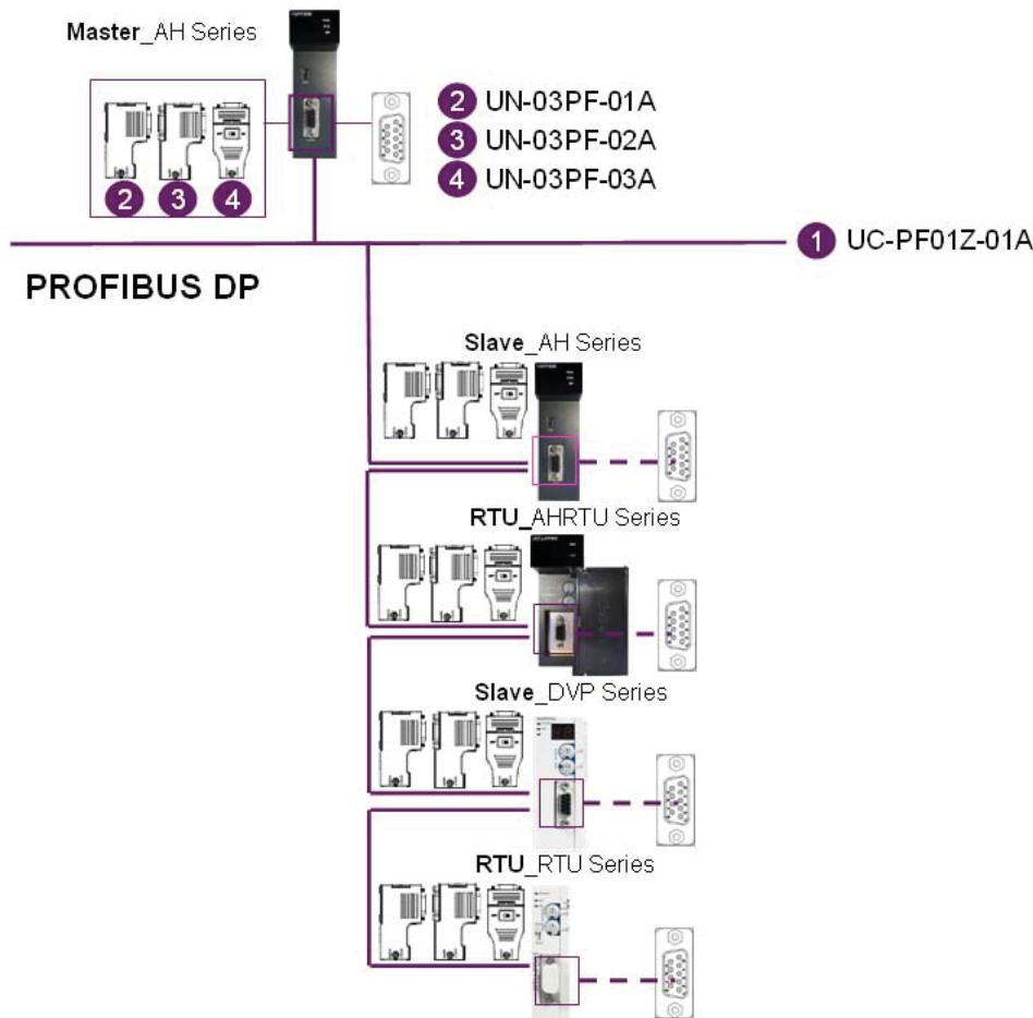
Note: If there are more than 32 pieces of hardware equipment in a network, or the communication length to which a communication rate corresponds is longer than the length specified (in the table below), the RS-485 repeater IFD5710 can be used to make the connection between cables longer.
