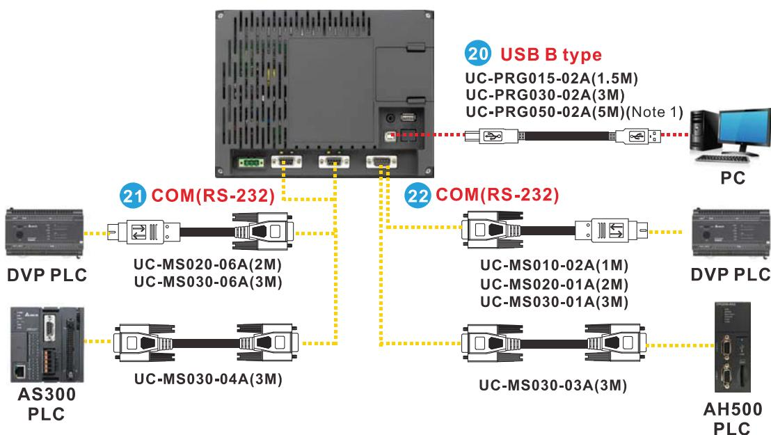
Note1: UC-PRG050-02A is used for transferring input signals between the interface panel and the controller. The cable is used exclusively for all-electric injection molding machines.
