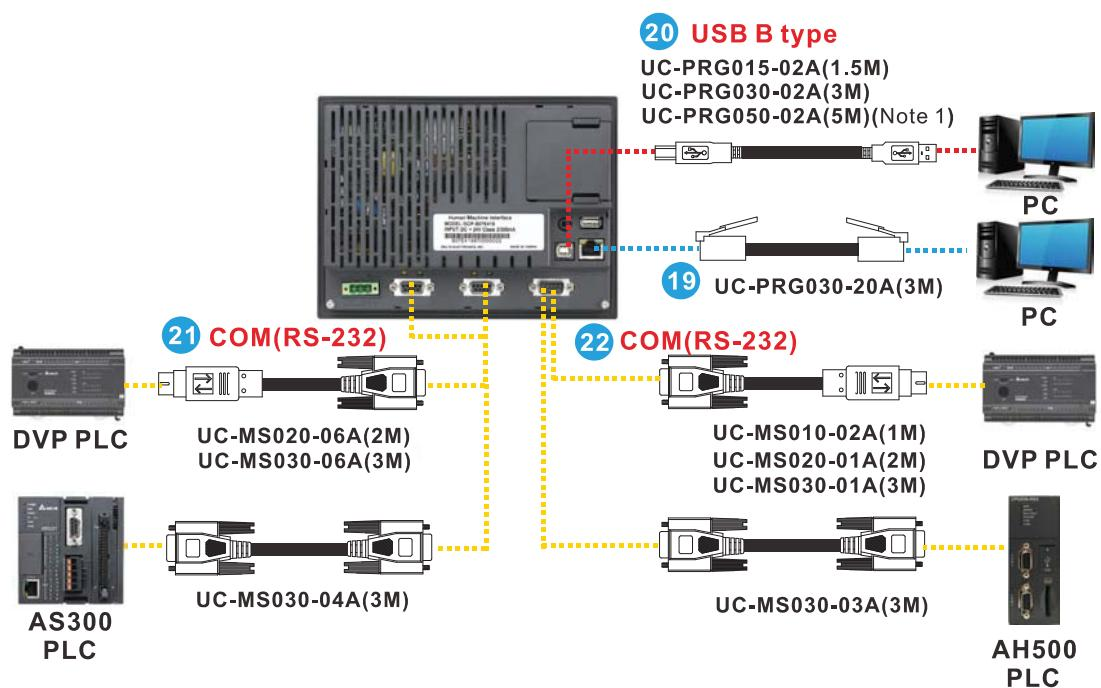
Note1: UC-PRG050-02A is used for transferring input signals between the interface panel and the controller. The cable is used exclusively for all-electric injection molding machines.
