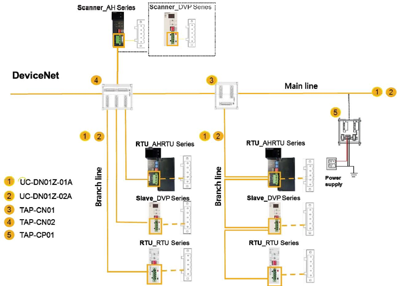
Note: DeviceNet requires that users connect a terminator to each end of a DeviceNet cable. The resistance of the terminators connected is  $121 \Omega$  (1/4 watts). Please refer to section 4.3.3 for more information about a terminator.
