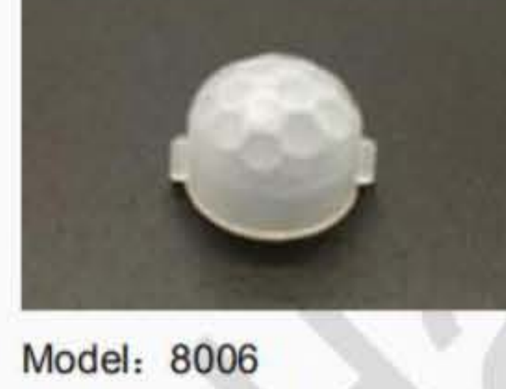
Model: 8006 Focal length: 7.5mm Angle: 120° Distance: 6m Size:ODφ15mmID:φ14mm
