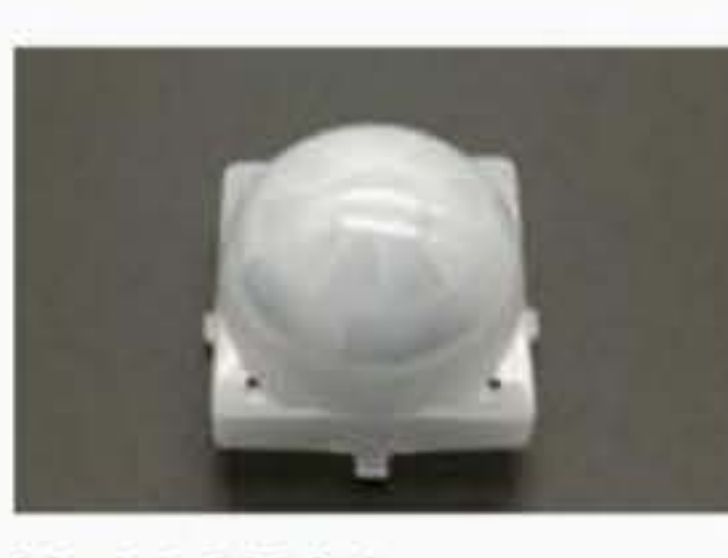
Model: 8002-1 Focal length: 10.5mm Angle: 100° Distance: 10m Size:φ23mm
