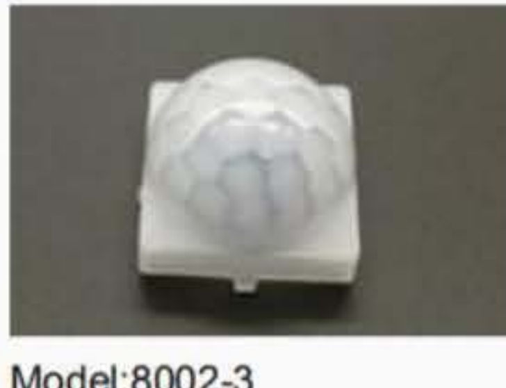
Model:8002-3 Focal length: 12mm Angle: 120° Distance: 10m Size:φ24mm
