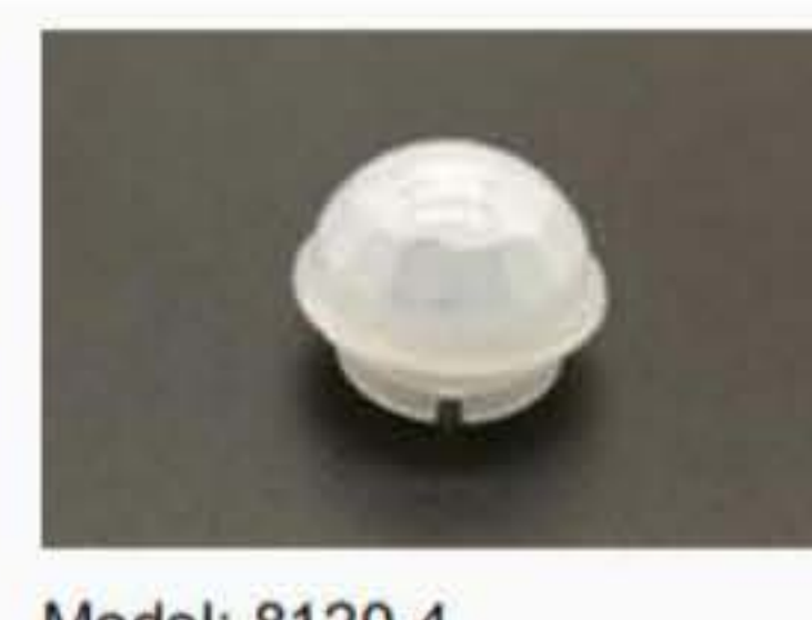
Model: 8120-4 Focal length: 6mm Angle: 120° Distance: 6m Size: φ12.7mm
