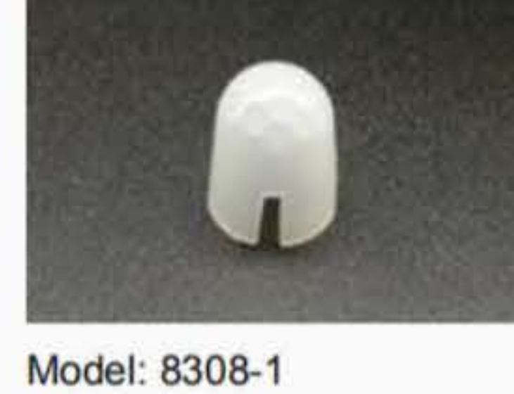
Model: 8308-1 Focal length: 6mm Angle: 60° Distance: 5m Size:φ11.5mm
