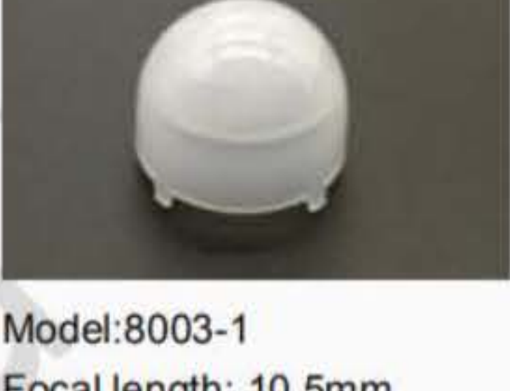
Model:8003-1 Focal length: 10.5mm Angle: 100° Distance: 7m Size:φ23mm
