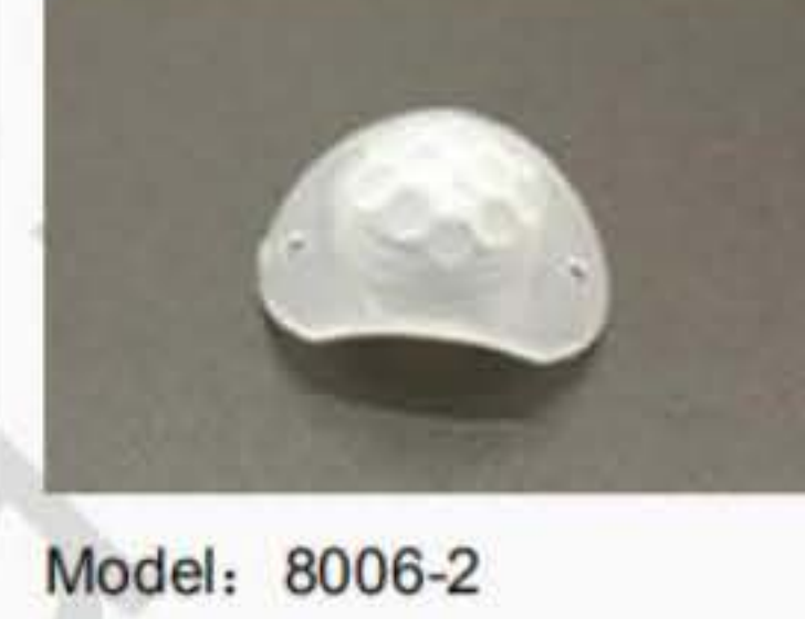
Model: 8006-2 Focal length: 4mm Angle: 100° Distance: 6m Size:φ17.1mm H:6.2mm
