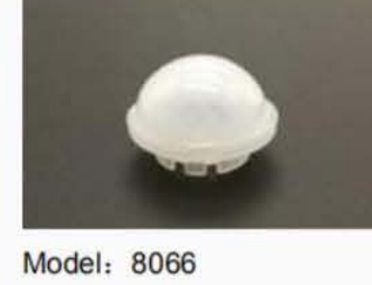
Model: 8066 Focal length: 7mm Angle: 60° Distance: 10m Size: φ16.5mm
