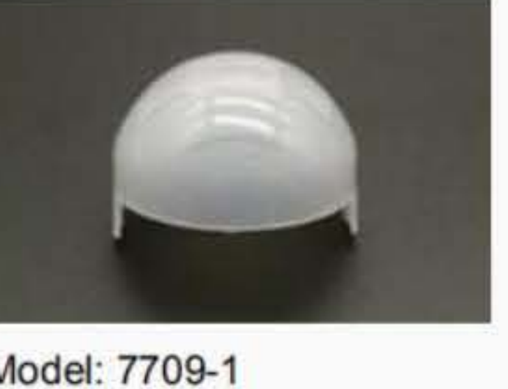
Model: 7709-1 Focal length: 7.6mm Angle: 90° Distance: 6m Size: φ21mm
