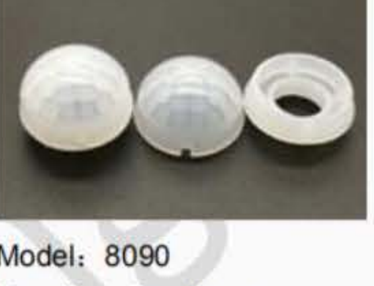
Model: 8090 Focal length: 9mm Angle: 120° Distance: 8m Size: φ17.8mm
