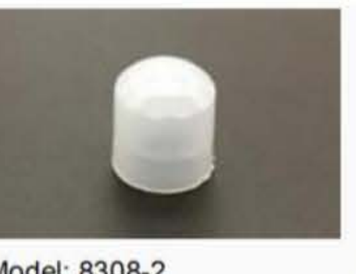
Model: 8308-2 Focal length: 9.5mm Angle: 80° Distance: 8m Size: φ12.5m high 14.3mm
