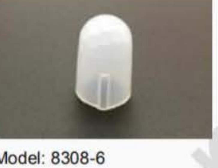
Model: 8308-6 Focal length: 9mm Angle: 90° Distance: 5m Size:φ11.51mmH: 16.61mm
