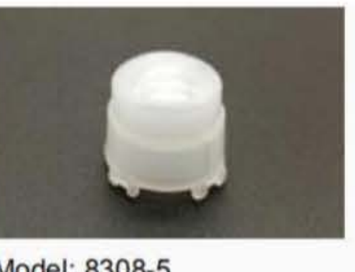
Model: 8308-5 Focal length: 9mm Angle: 90° Distance: 5m Size: φ10.27mm H:8.8mm
