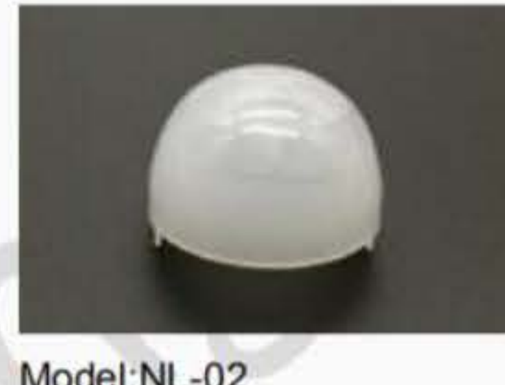
Model:NL-02 Focal length: 10.05mm Angle: 100° Distance: 10m Size: φ23.5mm H: 12.3mm
