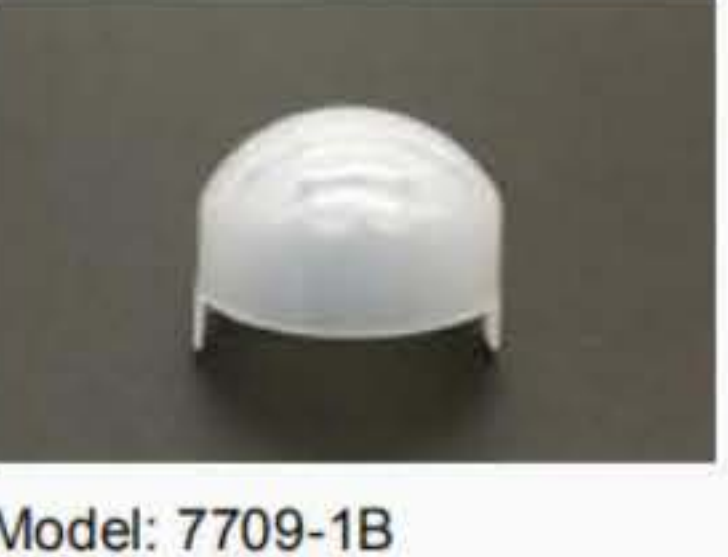
Model: 7709-1B Focal length: 7.6mm Angle: 90° Distance: 6m Size:φ20.7mm height 17mm
