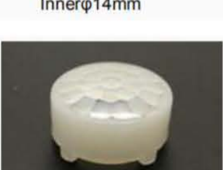
Model: 8225 Focal length: 15mm Angle: 120° Distance: 8m Size: φ22mm
