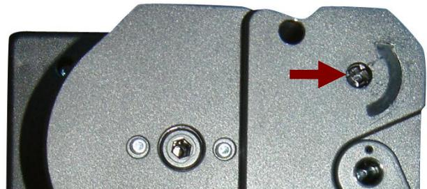
4. Turn the roller with the cross point tool **ANTICLOCKWISE** (as indicated by the arrow) until all the bank notes have been removed
