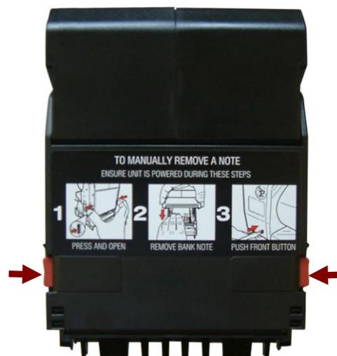
3. Carefully remove the bank note, then close the cover firmly and refit the module onto the validator head
