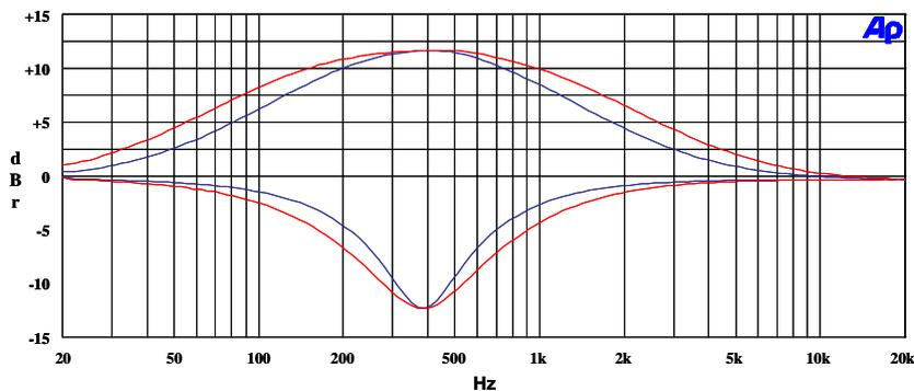
Figure 27: EQ Band 2, EQ2BW = 0 versus EQ2BW = 1
