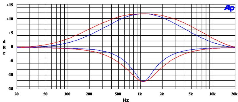
Figure 29: EQ Band 3, EQ3BW = 0 versus EQ3BW = 1
