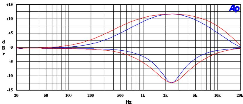
Figure 31: EQ Band 4, EQ4BW = 0 versus EQ4BW = 1
