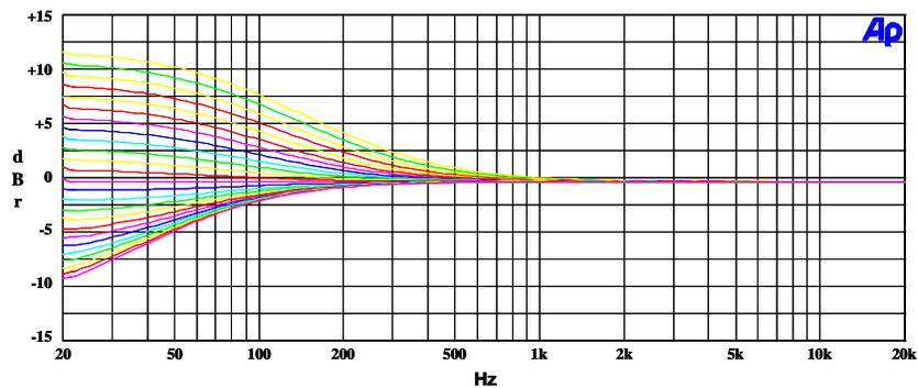
Figure 25: EQ Band 1 Gains for Lowest Cut-Off Frequency
