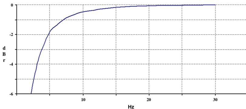
Figure 21: ADC Highpass Filter Response, Audio Mode
