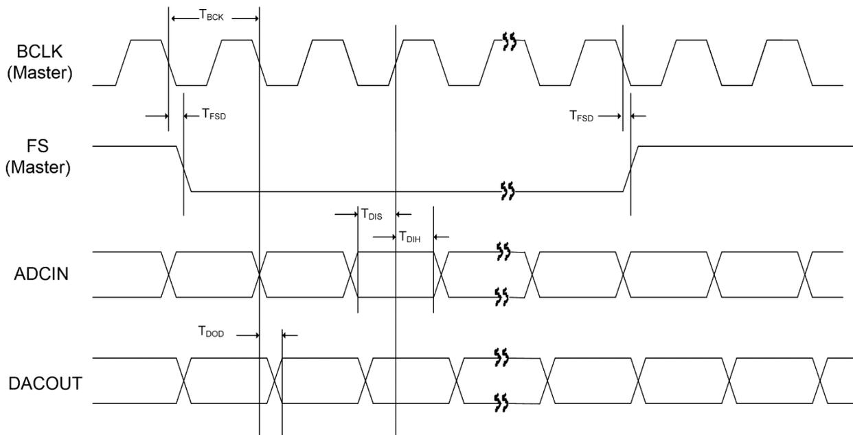
Figure 35: Digital Audio Interface Master Mode Timing
