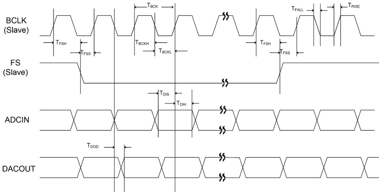
Figure 34: Digital Audio Interface Slave Mode Timing
