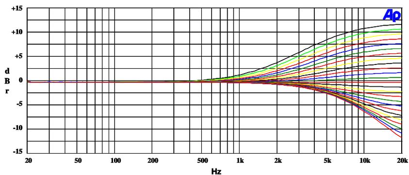
Figure 32: EQ Band 5 Gains for Lowest Cut-Off Frequency
