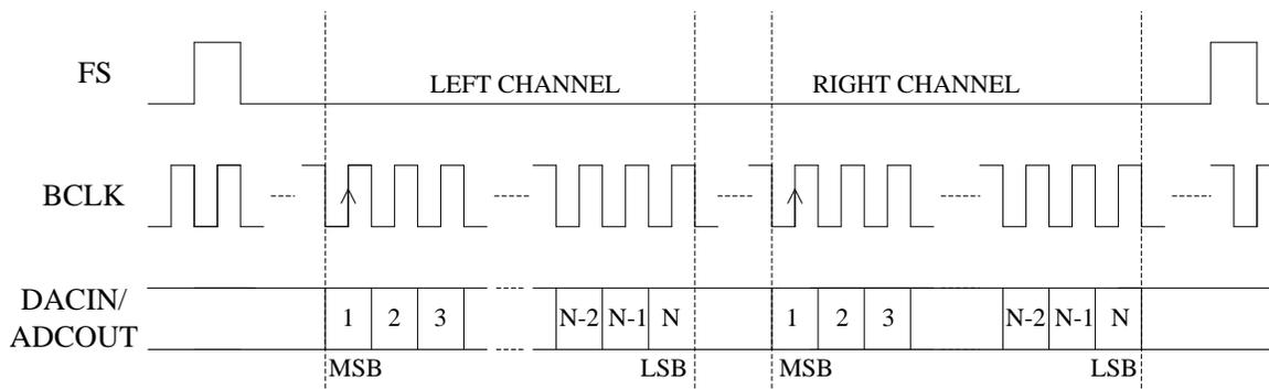
Figure 30: PCM Time Slot Audio Interface
